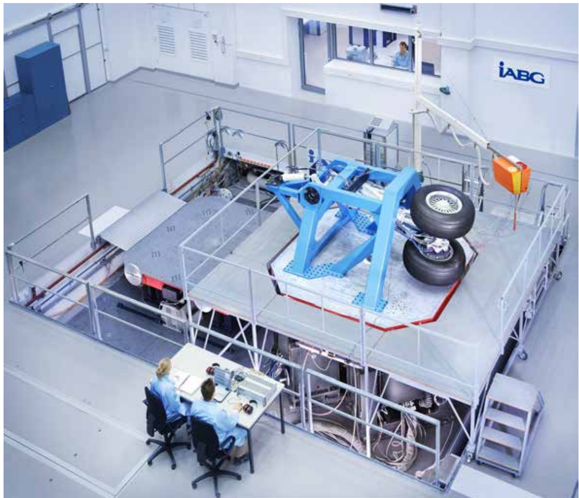
320 kN Multi-Shaker System with a main landing gear
