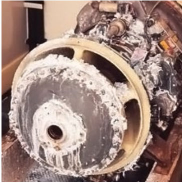
Corrosion test at a turbine
