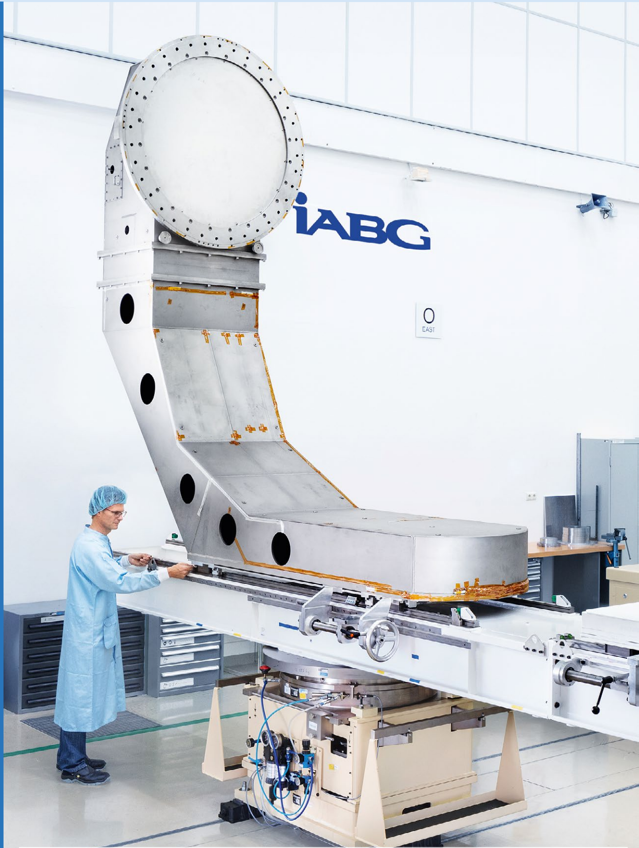
L-adapter for the determination of the centre of gravity and the moment of inertia
